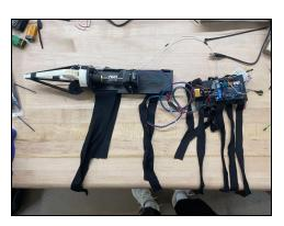
the actuation assembly and mounts to the patient's forearm) while the battery bay has its own platform on the shoulder of the user. The sensors and feedback circuit are comprised of the end effector's FSR for force control, an electromyography (EMG) sensor used to activate the device using the user's muscle electrical signals, and a vibration motor that will provide tactile feedback (to some extent [very limited one]) to the user.
